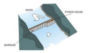
A series of integrated power developments along the same watercourse form what may be called a multistage hydroelectric system in which each portion of the river with a power plant of its own is referred to as a stage (Figure). The head created by a dam put across a lowland river usually ranges from 30 to 40m. In mountainous terrain, it may run over 200m.
