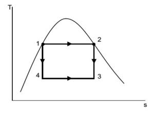
b)The carnot cycle is not a suitable model for vapour power cycle because it cannot be approximated in practice.
