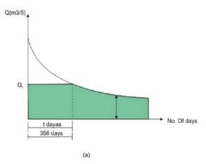
From this annual discharge curve, a truncation is made at a discharge Q which is the discharge corresponding to a time of
