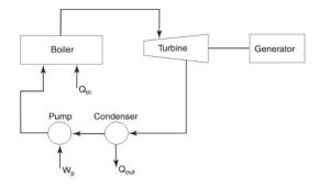
The schematic diagram also shows heat( $Q_{in}$ ) being supplied to the boiler and generator connected to the turbine for the production of electricity. Heat ( $Q_{out}$ ) is removed by the condenser and the pump supplies energy (Wp) to the feedwater in the form of a pressure increment to allow it to flow through the boiler.
